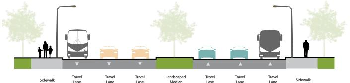
Example cross-section of arterial roadway with large right-of-way
