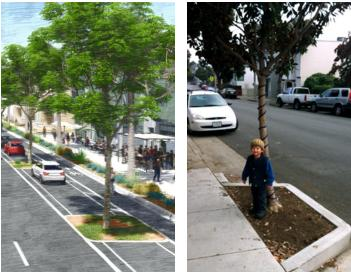
Parking lane planters can be a continuation of the sidewalk curb, or be constructed separate from the curb.
