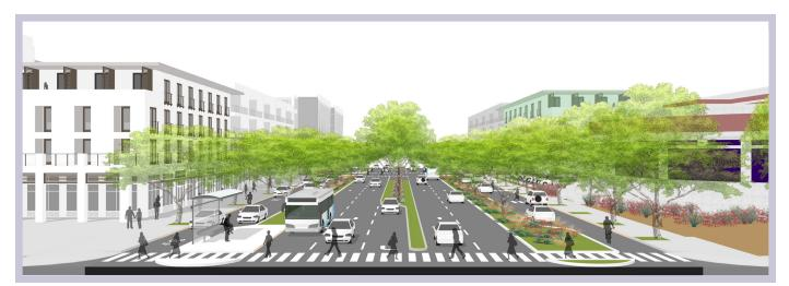
Alternative Frontage Lane Configuration: Curbside parking may be placed along the median to allow bulbouts near intersections. The bulbouts provide additional space for median refuge and for transit stops at median boarding islands.
