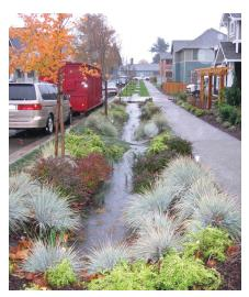
Bioswales help reduce stormwater runoff
