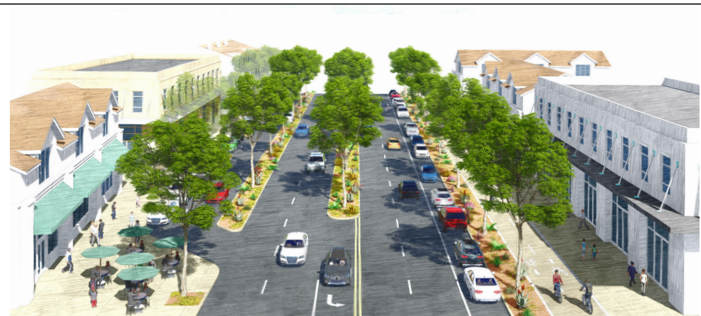
Vision for Foothill Boulevard entering into Rancho Cucamonga from the west. Streetscape improvements include widened sidewalks and a class IV cycle track on the south side of the street(right). A side access lane with curbside parking and wide sidewalks provide access to new mixed-use infill buildings to the north (left).
