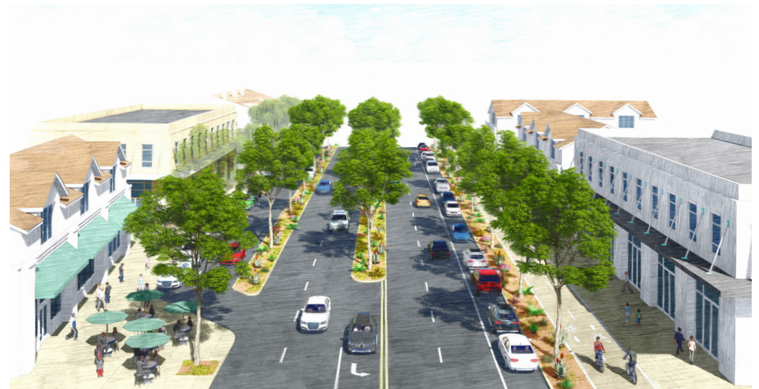
Vision for Foothill Boulevard entering into Rancho Cucamonga from the west. Streetscape improvements include widened sidewalks and a class IV cycle track on the south side of the street(right). A side access lane with curbside parking and wide sidewalks provide access to new mixed-use infill buildings to the north (left).
