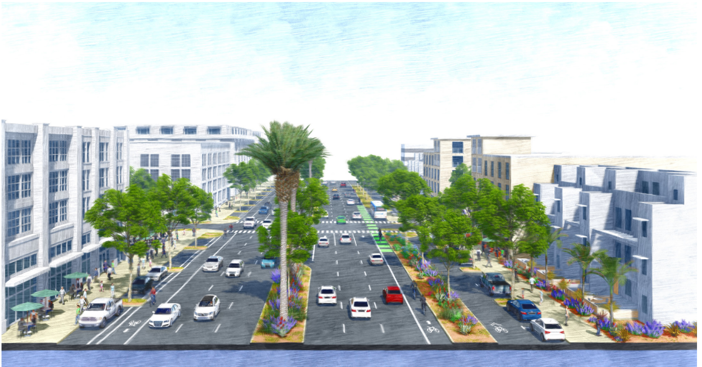
Foothill Boulevard improved with “bulb-in” parking on one side and a side access lane on the other in front of new mixed-use development
