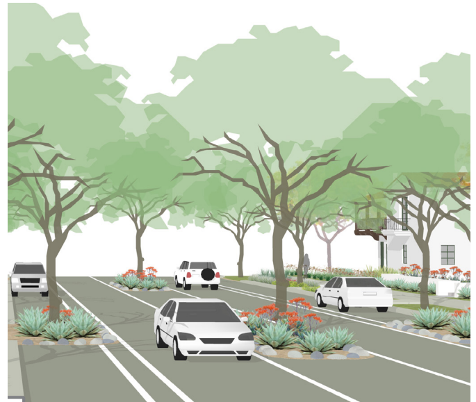
Where there are large roadways and curbside parking, medianettes can be designed in conjunction with parking lane planters.
