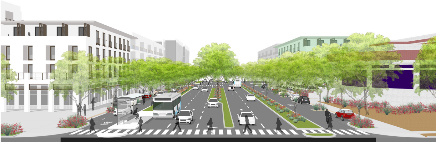
Phase 3: Convert protected bike lane into frontage lane with new curbside parking, street trees, landscaping, and enhanced sidewalk with the development of new street fronting commercial buildings.
