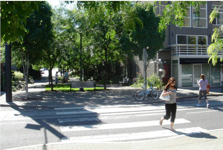
Mid-block crossing with zebra style crosswalk
