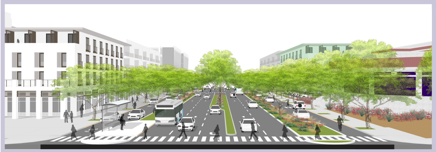
Alternative Frontage Lane Configuration: Curbside parking may be placed along the median to allow bulb-outs near intersections. The bulb-outs provide additional space for median refuge and for transit stops at median boarding islands.
