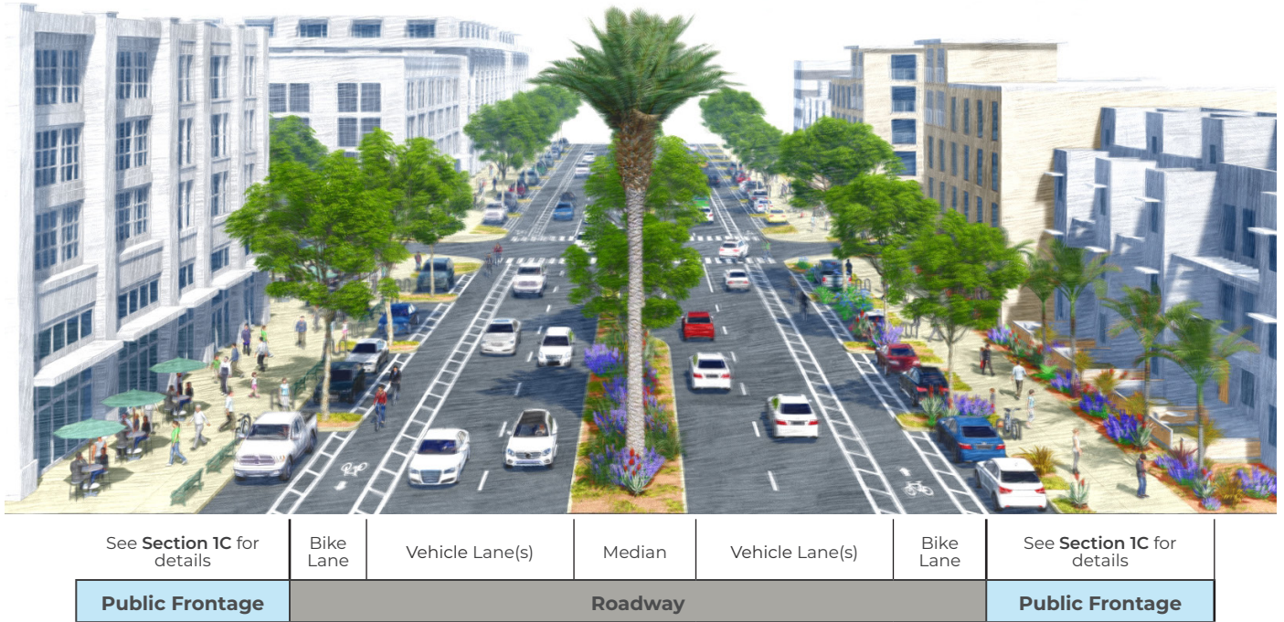
FIGURE PT-6 STREET RIGHT-OF-WAY COMPOSITION
