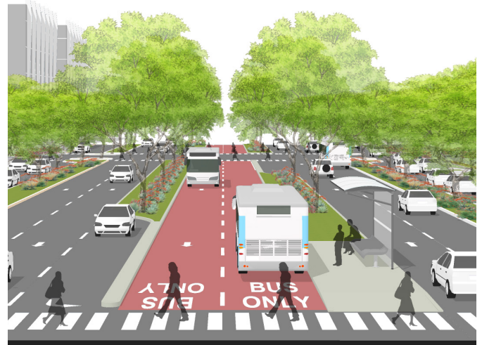
Center-running bus lanes with medians that accommodate transit stops and left turn lanes.
