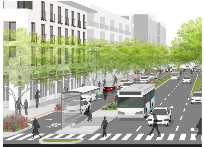
Peak-hour bus lanes may be integrated in streets with or without frontage lanes.
