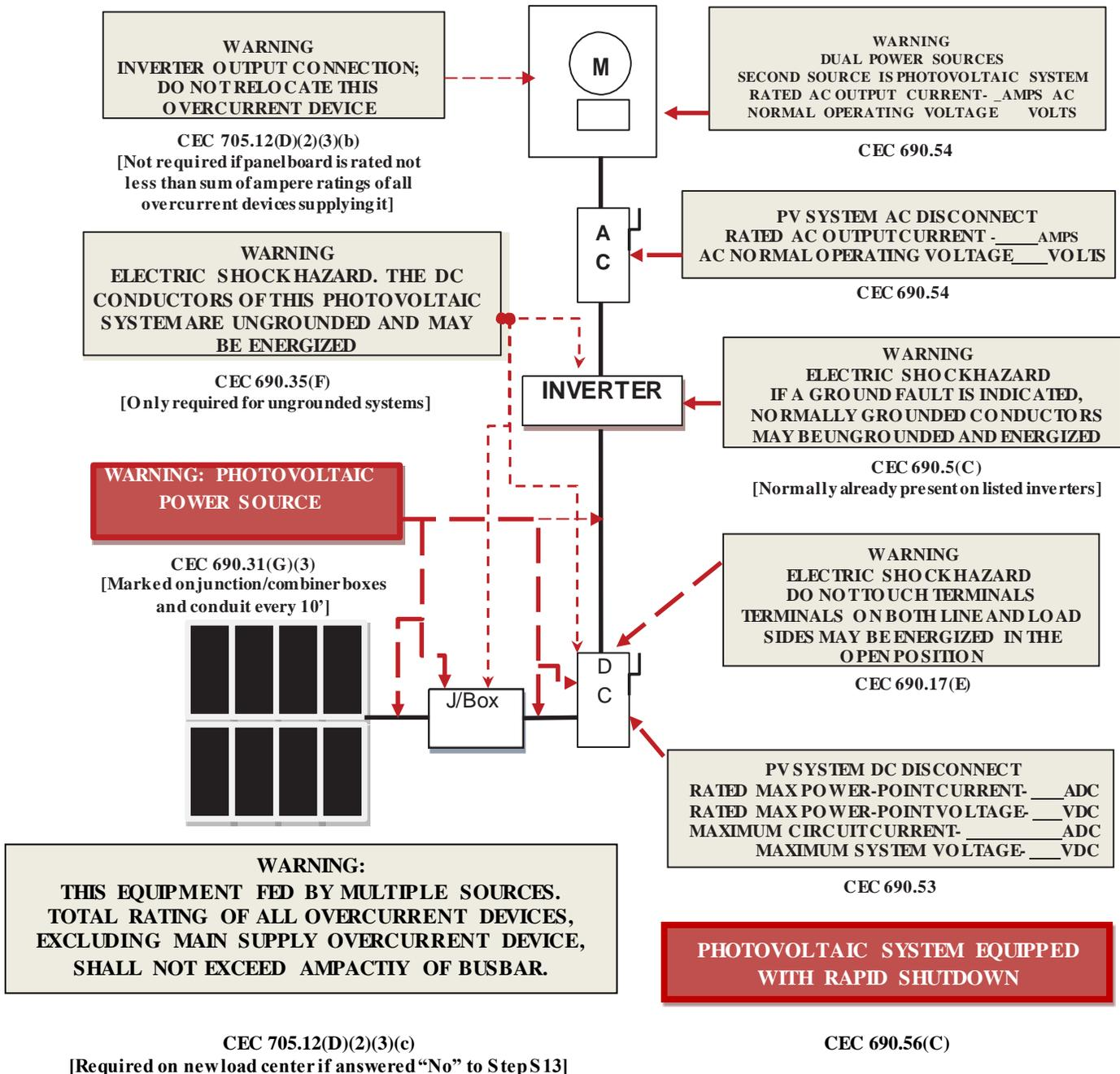
Informational note: ANSI Z535.4-2011 provides guidelines for the design of safety signs and labels for application to products. A phenolic plaque with contrasting colors between the text and background would meet the intent of the code for permanency. No type size is specified, but 20 point (3/8") should be considered the minimum.
